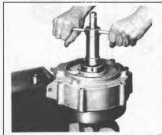
Figure 3-50. Pressing Flywheel into Crankcase
