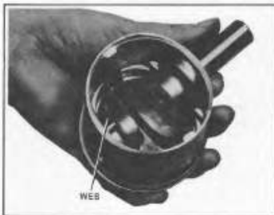
Figure 3-19. Piston with Web on Right Side
