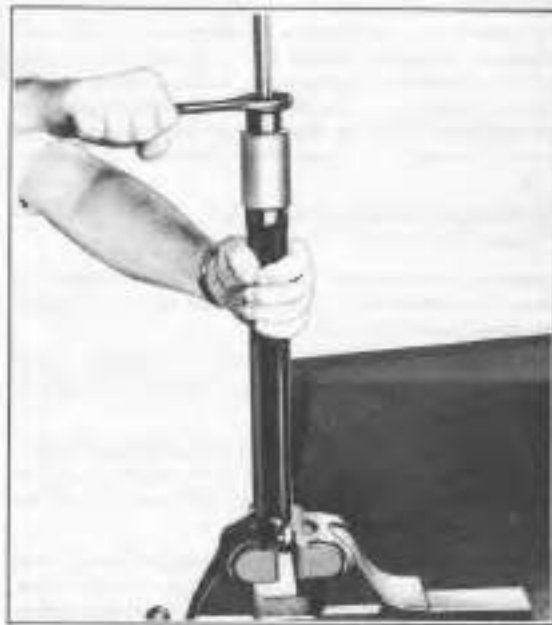
Figure 2-43. Removing Fork Slider Bushing
