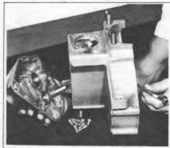
Figure 3-32. Line Reaming Cover Bushing
