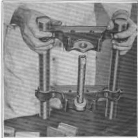
Figure 2-53. Checking Stem Alignment with Gauge
