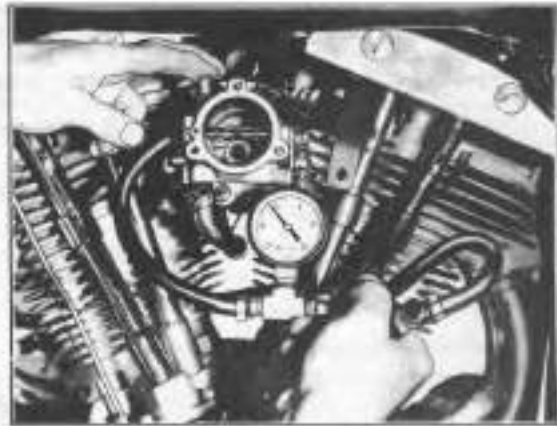
Figure 3-59 Checking Inlet Needle and Seat for Leakage
