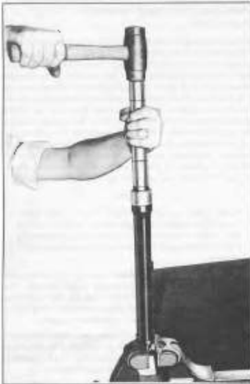
Figure 2-44. Reaming Fork Slider Bushing
