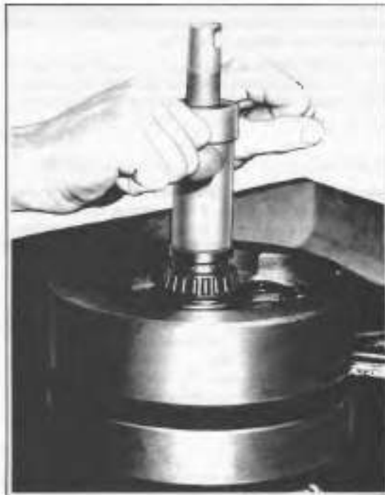
Figure 3-49. Pressing Bearing on Sprocket Shaft
