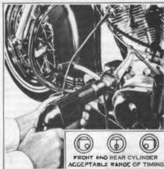
Figure 5-19. Checking Timing with Strobe Light
