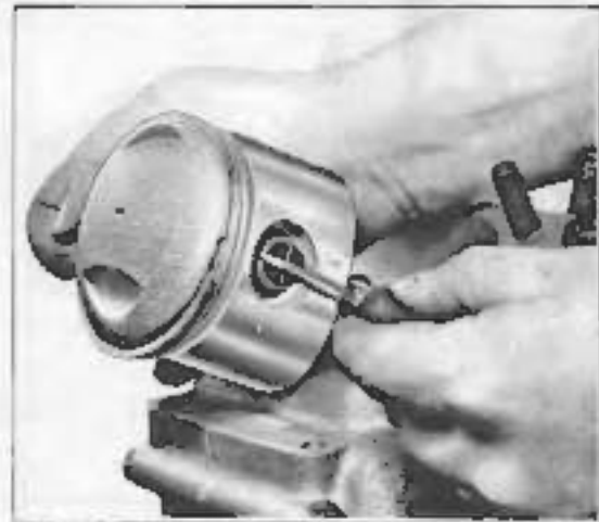
Figure 3-9. Removing Piston Pin Lock Ring (1972 and Earlier)
