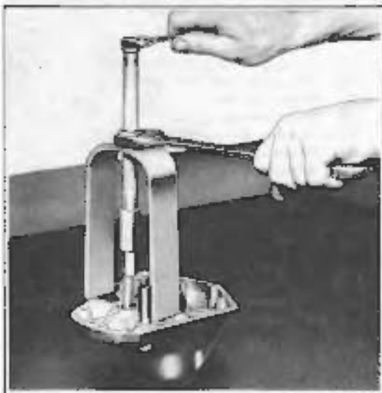
Figure 3-31. Removing Pinion Shaft Cover Bushing
