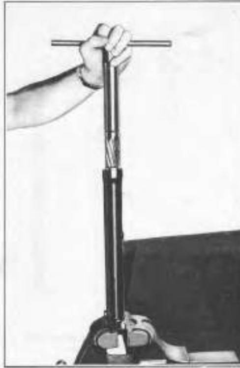
Figure 2-45. Reaming Fork Slider Bushing
