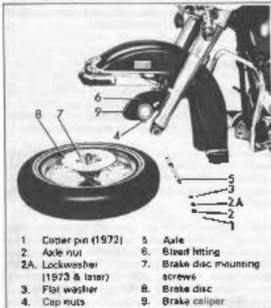
Figure 2-6 Front Wheel - FL (1972 and Later)
