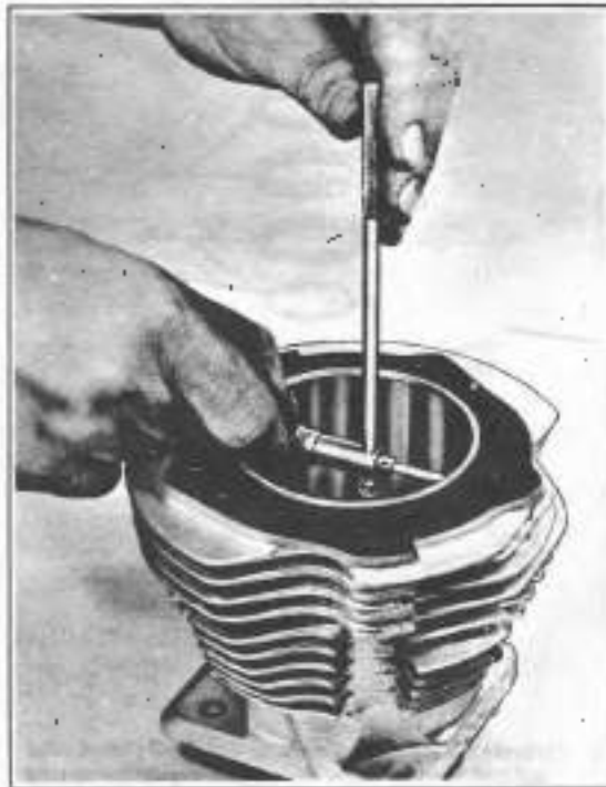
Figure 3C-4. Measuring Cylinder Bore
