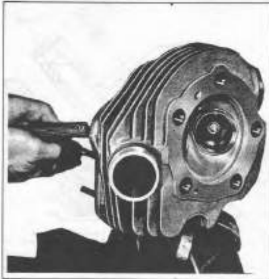
Figure 3B-4. Lapping Valves
