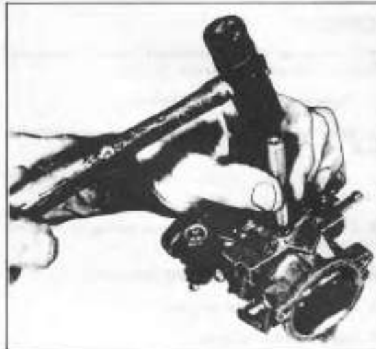
Figure 3F-7D. Removing Main Nozzle
