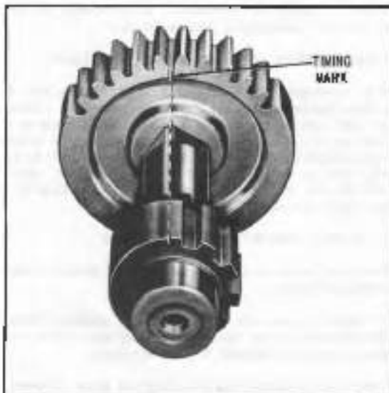
Figure 4D-7. Timing Shifter Gear
