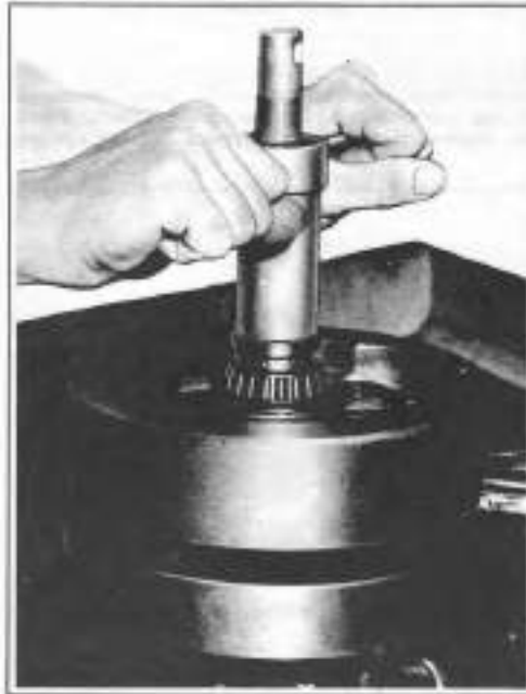
Figure 3E-15. Pressing Bearing on Sprocket Shaft
