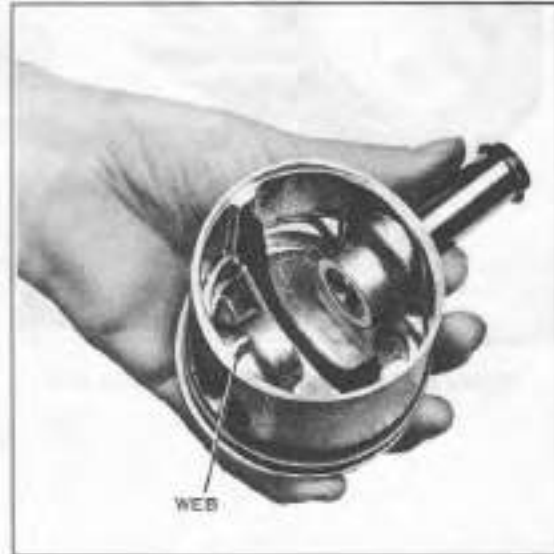
Figure 3C-13. Piston with Web on Right Side
