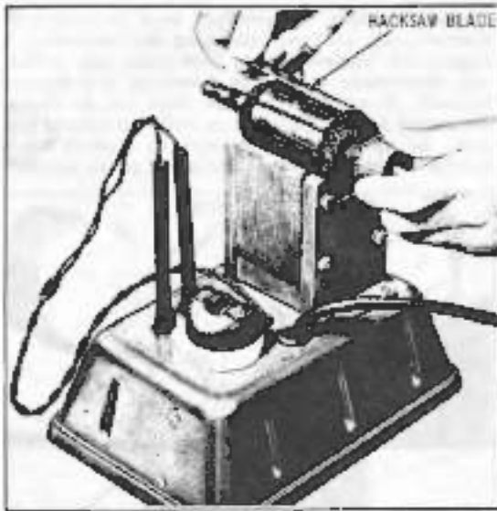
Figure 5E-4. Testing Armature for Short
