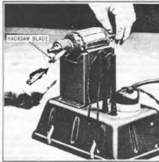
Figure 5E-5. Testing Armature for Open Circuit
