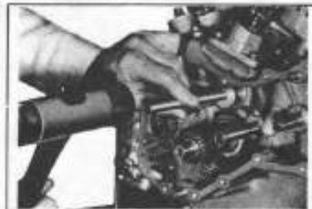
Figure 3D-9. Installing Cam Gear Needle Bearing in Crankcase
