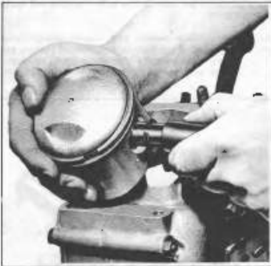
Figure 3C-14. Inserting Piston Pin Lock Ring
