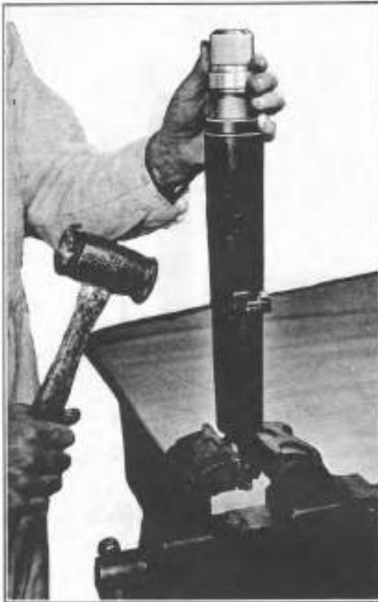
Figure 2F-11. Inserting New Oil Seal
