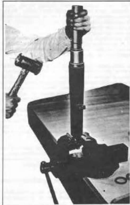
Figure 2F-7. Driving in Fork Slider Bushing
