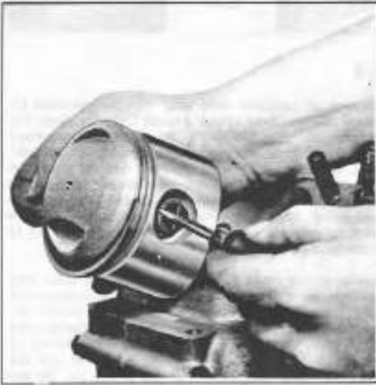
Figure 3C-2. Removing Piston Pin Lock Ring
