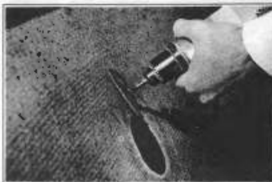
Figure 2J-8. Rough Sanding Inside Surface
