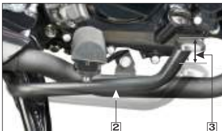
(2) Integrated/Rear brake pedal (3) Free play: 20–30 mm
