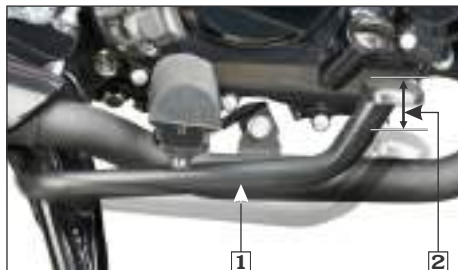
(1) Rear brake pedal (2) Free play: 20–30 mm
