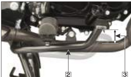
(2) Integrated/Rear brake pedal (3) Free play: 20-30 mm
