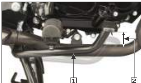
(1) Rear brake pedal (2) Free play: 20-30 mm
