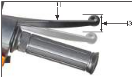
(1) Front brake lever (3) Free play: 10-20 mm
