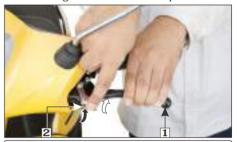
(1) Integrated brake lever (2) Lever lock
