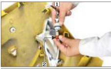
(1) Bulb holder (2) Front turn signal bulb
