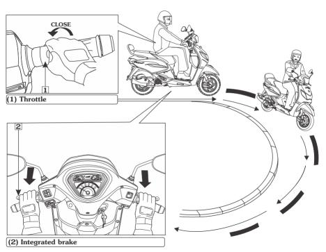
• When descending a steep gradient, Avoid continuous use of the brakes, which close throttle (1) fully and apply integrated brake (2) to slow down the vehicle.
