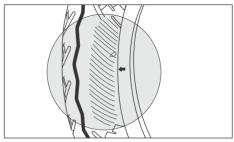
• Carefully inspect the tyres for any damage, if the vehicle hits a pothole or hard object.
