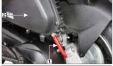
(1) Drain tube (2) Air cleaner assembly
