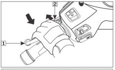
(1) Integrated brake lever (2) Lever lock
