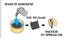
Squeeze it in a manner so that oil will spread on complete surface of pre foam element.
