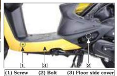
To dislodge the tabs (4), slide the floor side covers to the rear side and pullout the floor side cover.
