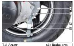
If the arrow aligns with the reference mark on \*MF stands for Maintenance Free full application of the brake, the brake shoes must be replaced. Visit your Authorised Hero MotoCorp workshop for this service.
