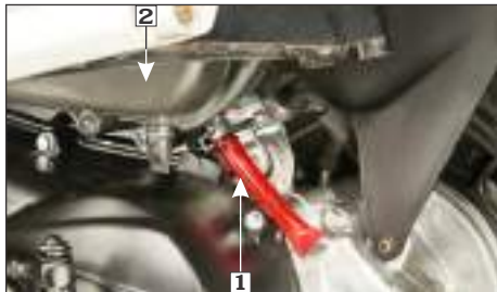
(1) Drain tube (2) Air cleaner assembly
