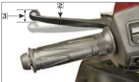
(2) Integrated brake lever (3) Free play: 10-20 mm
