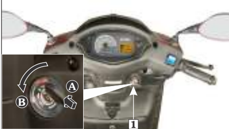
(1) Ignition switch (A) Push in (B) Turn to lock
