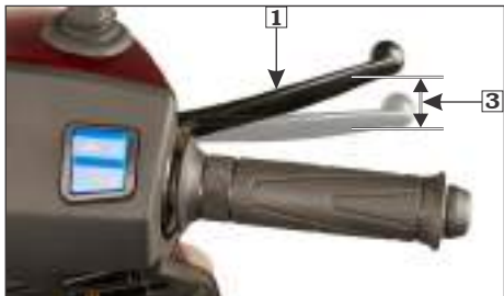
(1) Front brake lever (3) Free play: 10-20 mm
